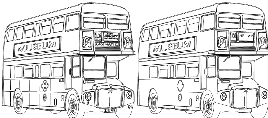
Figure 5.7: Left: a wire model of the original image, Right: a wire model of the image after the RemoveSmallPrimitives method
